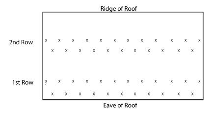
Above example is based on Metal Roof Panels being 36" Panels with 9" rib spacing.
